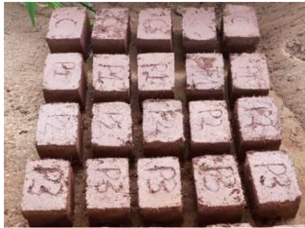
Fig. 3. Photograph showing freshly moulded block specimen
