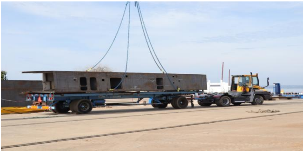
Fig. 13. Transportation of sections from fabrication yards
