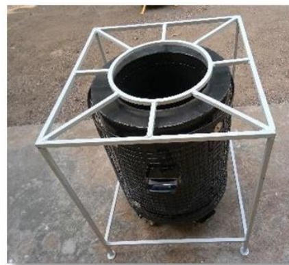
Fig. 2. Top view image of Dhaba-sized cook stove system
