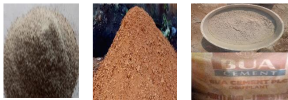
Cattle bones Ash (after grinding and calcination) Laterite soil in the study area ordinary cement product, (BUA Nigeria) Portland cement (BUA)
