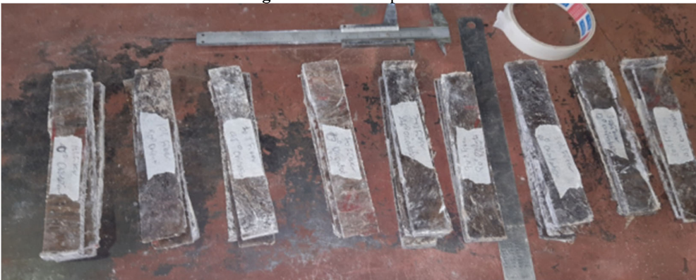
Fig. 8. Flexural test specimens
