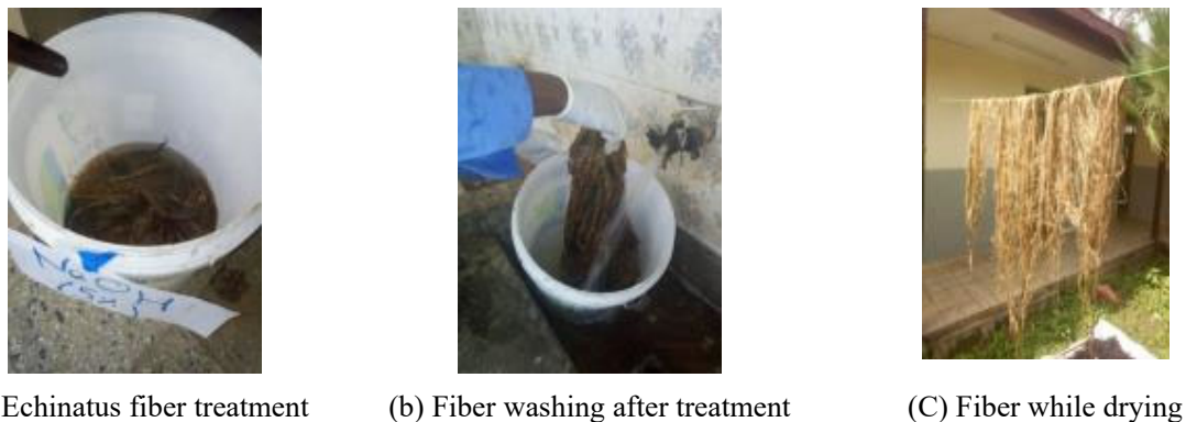
Fig. 3. Echinatus fiber treatment and drying process
