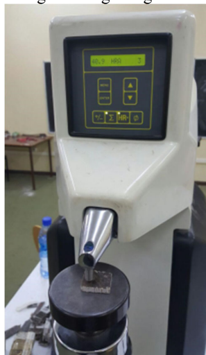
Fig. 12: Specimen under hardness test
