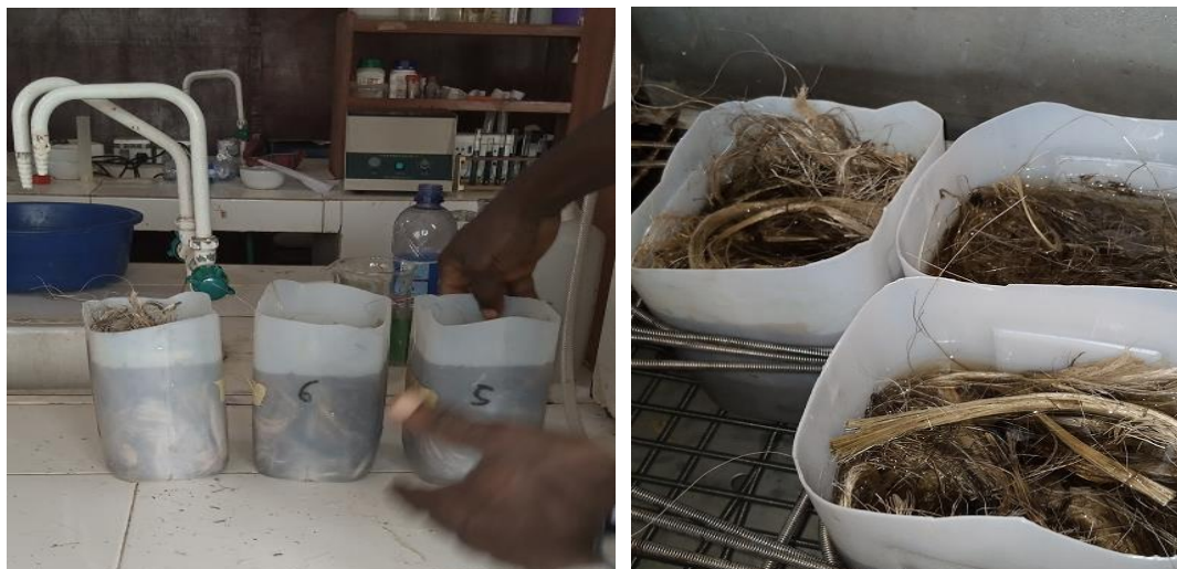
Fig. 1. NaOH treatment of fibres
