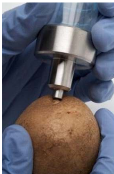
Fig. 2. Potato coring device (Courtesy of J. Smith, Fera Science Ltd, York, UK)
