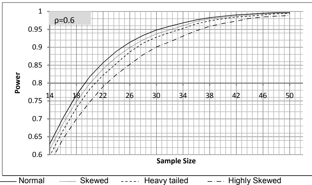
Fig 6. Power curves of correlation test for \rho= 0.6 when the bivriate distribution of population is normal, skewed, heavy tailed and highly skewed
