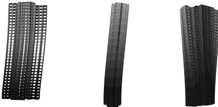
Fig. 14 a. The first-order translational mode b. The second-order translational mode c. The third-order rotational mode
