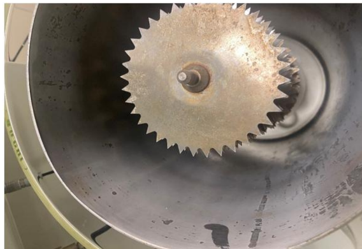
Fig. 3. Buchi Spray Dryer Particle Collector showing particle sticking
