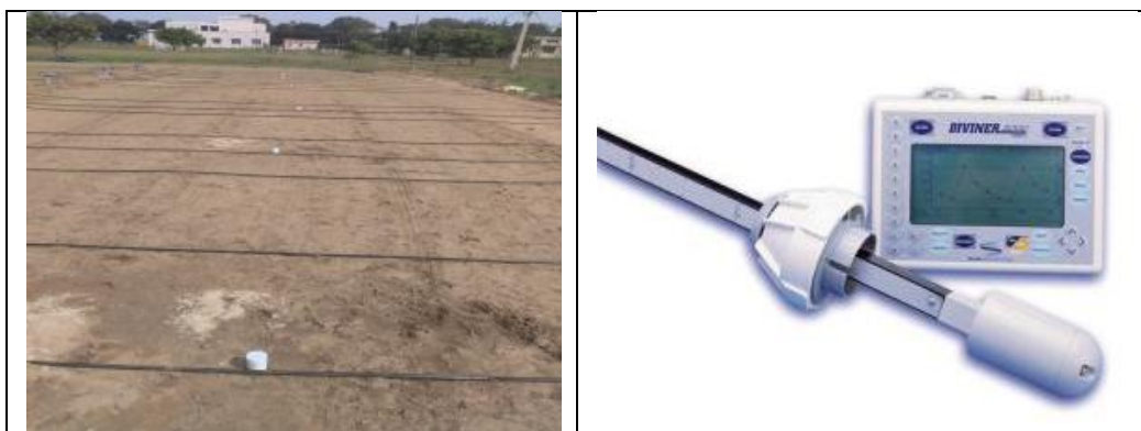
Plate 2. Installed access tubes and FDR sensor
