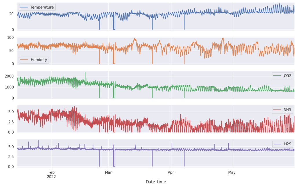
Figure 7. Fattening data collected indoors from a pig farm environment includes measurements of temperature, humidity, \text{CO}_2 , \text{NH}_3 , and \text{H}_2\text{S} .
