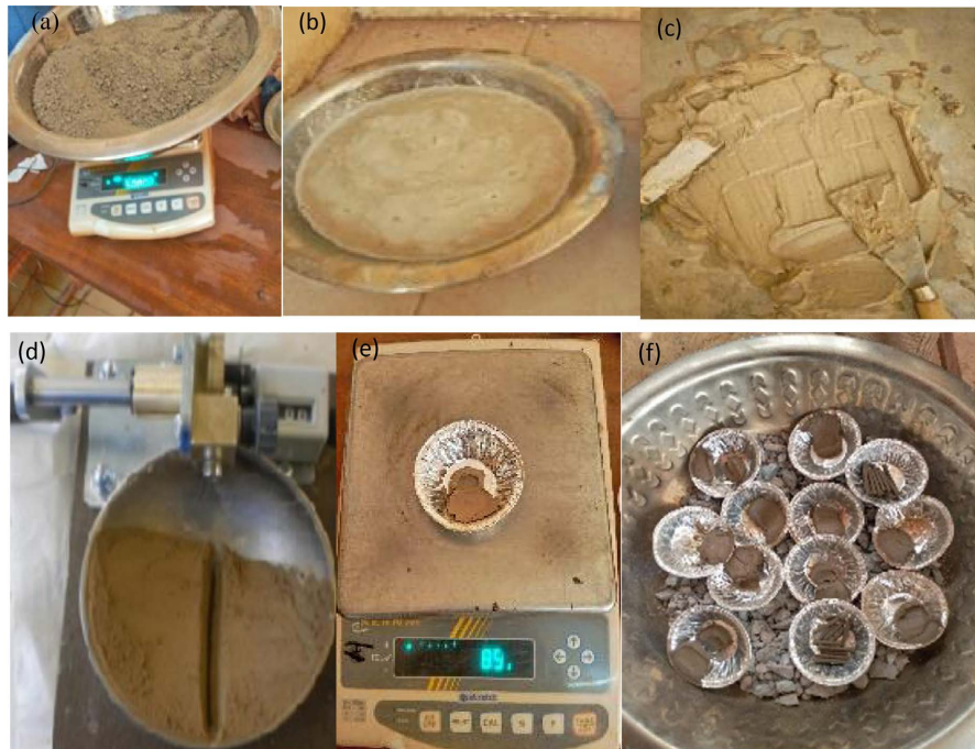
Figure 2. Procedure for Determining Limits: (a) Sampling, (b) Settling, (c) Kneading of the Passing, (d) Sampling of the Kneaded, (e) Weighing, and (f) Recorded Tare.
