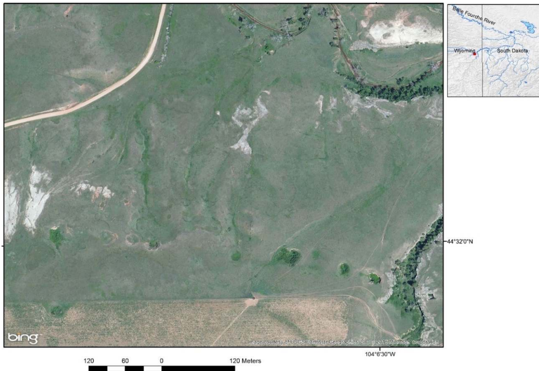
Fig. 16. Dolines tracing linear subsurface structures as visible on a BingMaps_Aerial-scene
