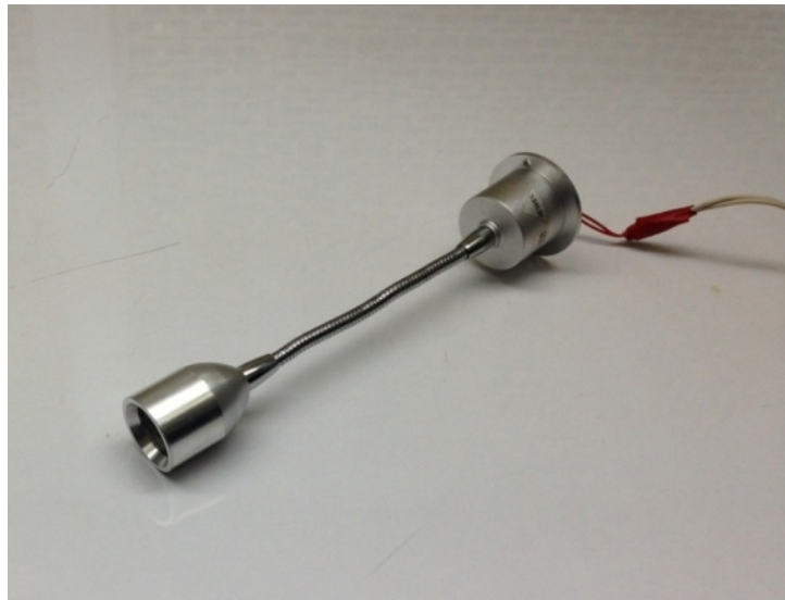
Fig. 2. The LED used in this experiment: XR-C, Cree Inc., Germany, with a wavelength of 637 nm
