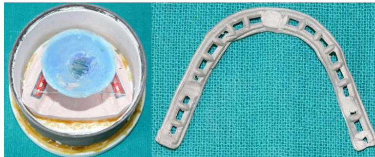
Fig. 6. Refractory cast with wax pattern and sprue attachment and finished metal framework
