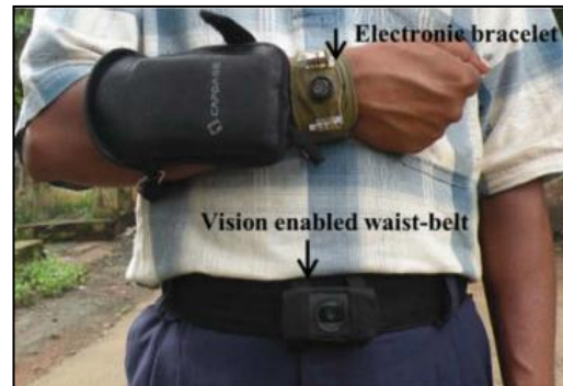
Fig. 6. A blind volunteer showing a typical posture for the use of the electronic bracelet and the vision-activated belt system (EBVEWB) [14]
