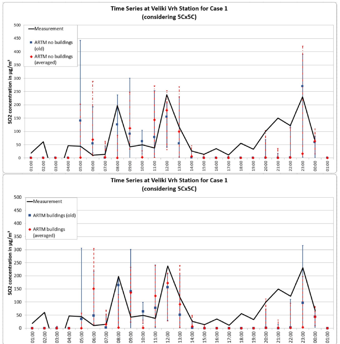
Figure 5. Measurements of \text{SO}_2 ( \mu\text{g m}^{-3} ) at the Veliki Vrh Station for the 30 March 1991 case (Case 1) compared with predictions from ARTM, both without accounting for buildings at the emission site (top) and with accounting for buildings at the emission site (bottom). The measurements have been averaged to show an hourly resolution. The error bars show the deviation range of the five-by-five cells target grid around the Veliki Vrh station to allow for slight deviations in the model predictions with respect to the location of the measurement points.
